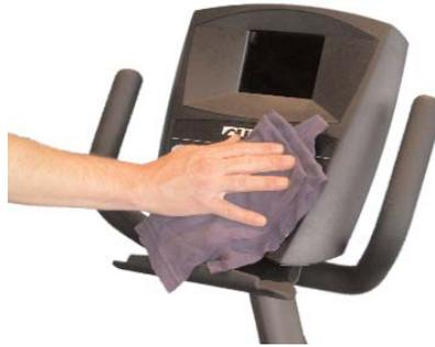
**Weekly.** Wipe down your Z8.1 Bike once a week with a water-dampened soft cloth. On the contact heart rate pads, use a glass cleaning solution. Be careful not to get excessive moisture between the edge of the overlay panel and the console, as this might create an electrical hazard or cause the electronics to fail.
